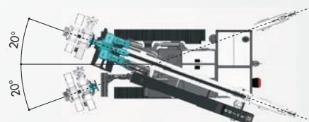
Rig movements are the maximum allowable. Any additional equipment on the rig may limit these movements.
